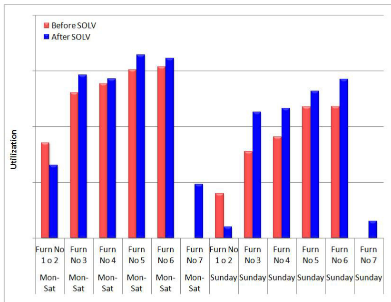
Fig. 2. The average utilization of the heat treatment resources has been significantly increased by the usage of the optimal scheduling tool SOLV. The averages 'After SOLV' have been calculated for the first 6 months of usage of SOLV, and the averages 'Before SOLV' have been calculated for the corresponding months the previous year.
